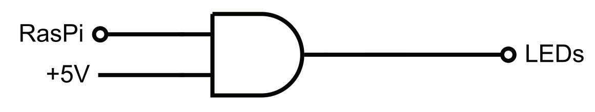
To build this sculpture we used 280 LEDs arranged in a helix structure with 14 bars each representing a different frequency. The LEDs are configured in two parallel strips running in parallel across the helix that allows for a synchronized visualization. Because the strips require 5 volts but the Raspberry Pi only outputs 3.3 volts we used an And Gate to convert to the correct voltage.
